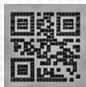
Micro QRcode ( 750\mu\text{m} \times 750\mu\text{m} )
